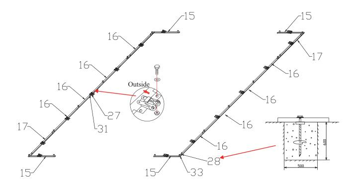
Step 2: Install the first row of rafters with #1,#2,and #3,#5,#6, then put it in the base feet.(To avoid accident, It is very important to hold the first row of rafter with support(wood, rope or similar thing), make sure that it won't fall down.)
