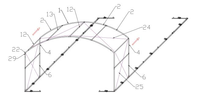
Step 3:Install the second row of rafters with #1,#2 and #4, #6, Put it in the base feet, then connect to first row with #12,#13,brace with #24,#25 and fasten.
