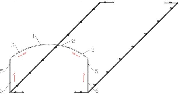
Step3:Install the second row of rafter with #1,#2 and #4,#6, crane/lift into base feet,then connect to the first row with #12,#13. And brace with #24,#25.
