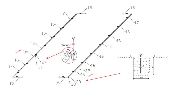
Step 2: Install the end rafter with #1,#2 and #3,#5,#6,crane lift it into base feet. (To avoid accident, It is very important to hold the first row of rafter with support (wood, rope or similar stuffs), make sure that it won't fall down.)
