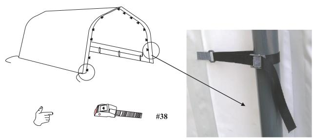
Note:#38for main roof cover tensioning. #39 for front and end covers tensioning.
