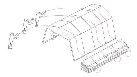
insert the conduit to pocket on side:
