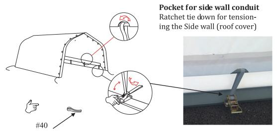
Step 2: Attach the cover (#35/#36) to the frame as following:
