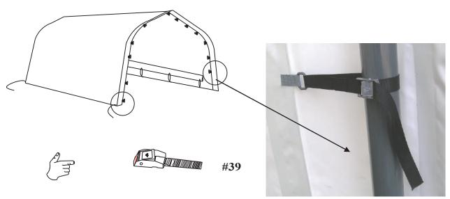
Note:#39 for main roof cover tensioning. #38 for front and end covers tensioning.
