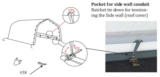
Step 2 : Attach the cover to the frame as following :
