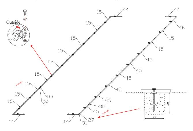
Step 2: Install the end rafter with #1,#2 and #3,#4,#5,crane/lift it into base feet. (To avoid accident, It is very important to hold the first row of rafter with support (wood, rope or similar stuffs), make sure that it won't fall down.)
