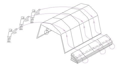
insert the conduit to pocket on side:
