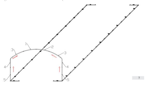
Step3 :Install the second row of rafter with #1,#2 and #4,#5, crane/lift it into base fee, then connect to the first row with #11,#12, and brace with #24,#25.
