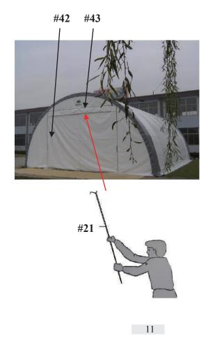
(in order to protect the shelter from heavy wind, please install the wind bracing straps at points 300 mm measuring from the ends, and others to be installed in the middle averagely.) (photos are for reference only, the real quantity is according to packing list.)
