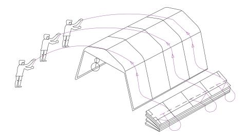
insert the conduit to pocket on side:
