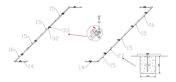
Step 2: Install the first row of rafters with#1,#2,and #3,#4,#5,then put into base feet,(It is very important to hold the first row of rafter with wood, rope and etc to avoid the hurts and damage of falling down.)
