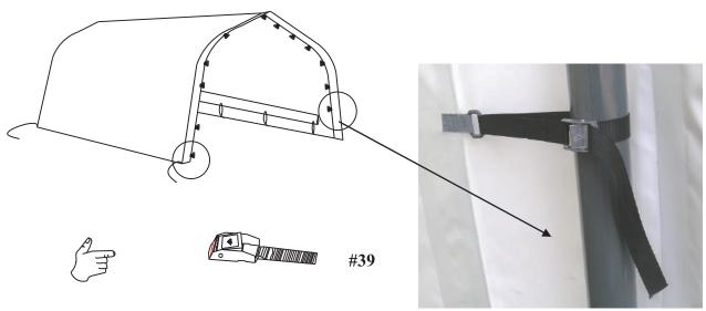
Note:#39 for main roof cover tensioning. #40 for front and end covers tensioning.
