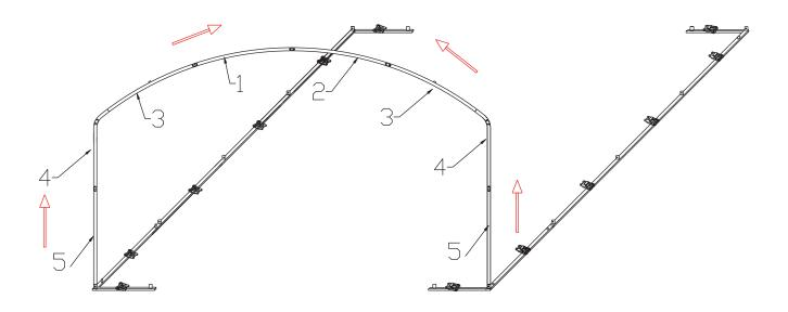
Step 3:Install the second row of rafter with #1,#2 and #4,#5, put into the base feet, then connect with first row with #11 and #12, brace them with #24,#25.
