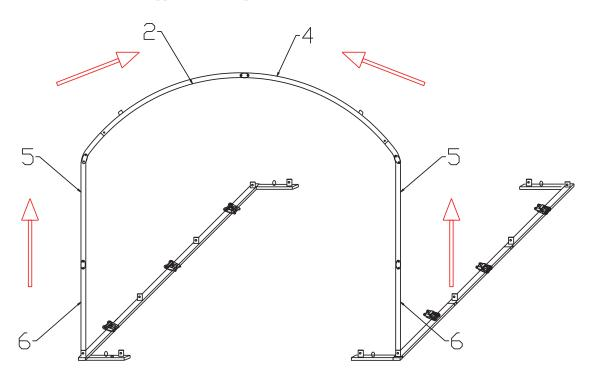
Step 3:Install the second row of rafters #1, #3 and #5, #6, put into feet and connect with end rafters with #11, #12, then brace with #24,#25.
