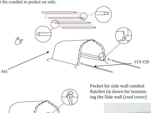
Step 2: Attach the cover (#35/#36) to the frame as following:
