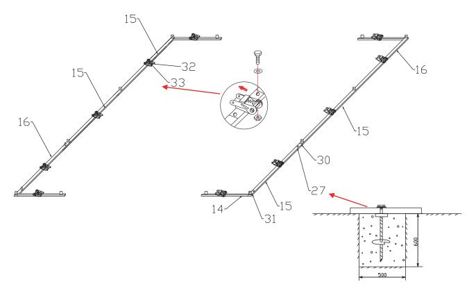
Step 2: Install the end rafters #2,#4 and #5,#6 (To avoid accident, It is very important to hold the first row of rafter with support (wood, rope or similar stuffs), make sure that it won't fall down.)
