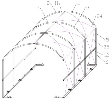
Step5: Install the door frames as illustrated below, then fasten all the screws and parts.
